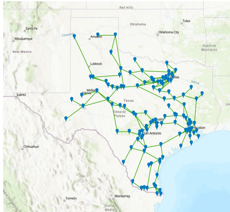
Fig. Texas 123-bus transmission network topology.
