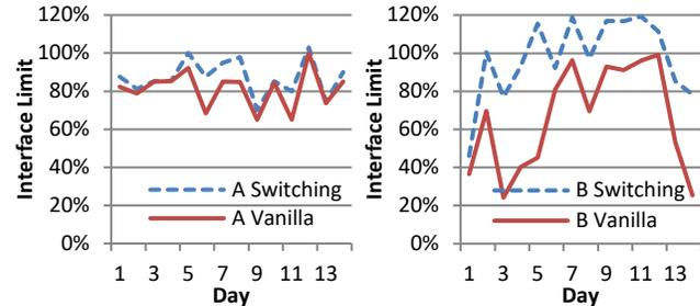
Fig. 9. Interface limit improvements with corrective switching. The values are normalized by the largest limit observed over the study period.
