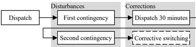
Fig. 3. The N-1-1 process and where corrective switching may be added.
