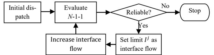
Fig. 4. The iterative process to calculate the limit for interface  $j$ . The evaluation of N-1-1 reliability simulates the steps in Fig. 3.
