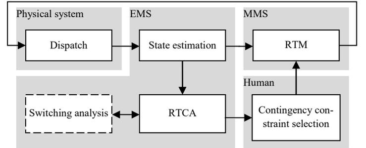
Fig. 2. Summary of real-time operations relevant to this study. This study simulates the RTCA, switching analysis, and the RTM. All other steps are replaced by historical data.
