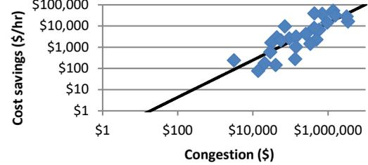
Fig. 7. Relationship and regression fit for cost savings vs. congestion  $\tilde{\alpha}$ . Note the scale is log-log.
